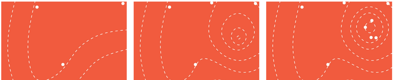
△ Figure 5. Diagram of three iterations of a global, model-based algorithm. The dashed lines indicated the approximated design space.
